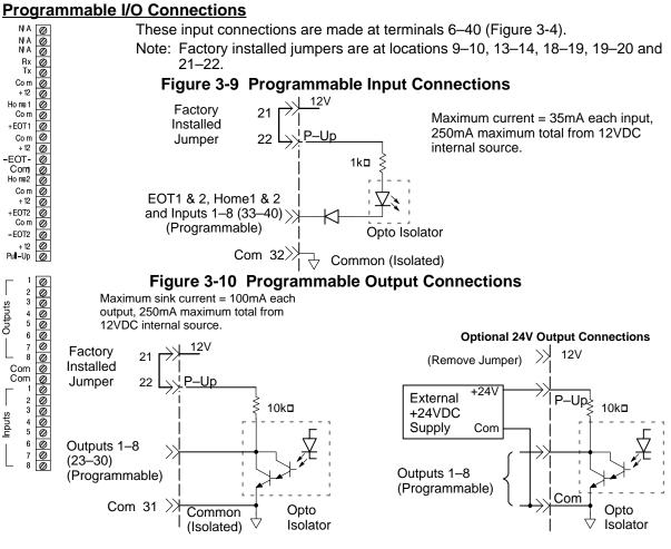
Factory installed jumper for 12VDC pull–up operation. Maximum current sink capability is 100mA per output and 350mA maximum from internal 12VDC supply.
